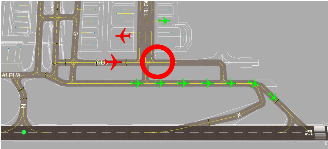
Figure D.12: Code E Arrival Bypassing Departure Queue on Second Parallel Taxiway
